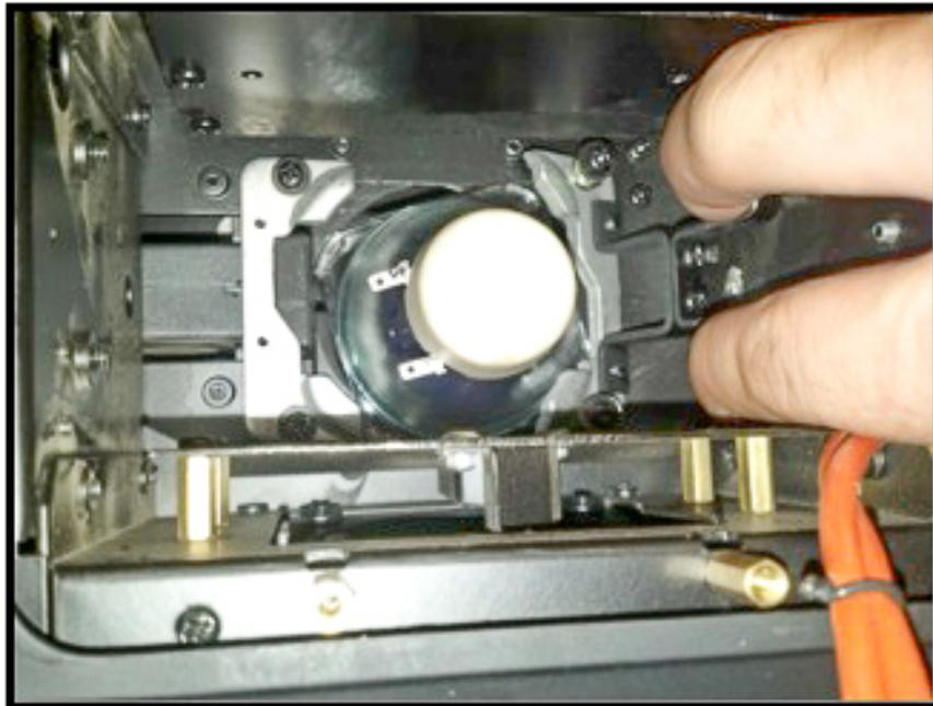
7. While still holding the retention handle with your **RIGHT** hand, gently turn the lamp **CLOCKWISE** with your **LEFT** hand until the lamp is correctly aligned under the retention brackets.
